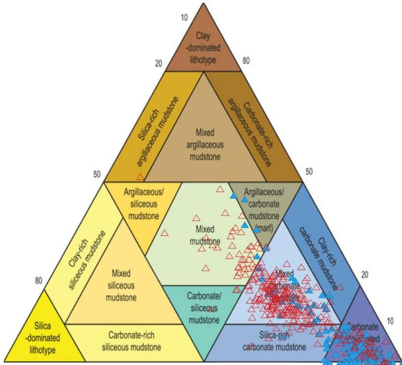
Figure 2. Ternary diagram from Schlumberger for mudrock lithofacies classification based on dry weight components of clay, carbonate, and quartz-feldspar-mica (QFM). Eagle Ford (red triangles) samples are characterized as mixed carbonate mudstones and the Austin Chalk (blue triangles) is classified as a carbonate dominated lithotype.
