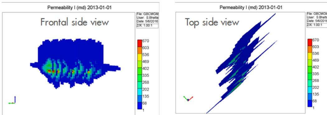
**Figure 1. Realistic fracture model that can be imported into the reservoir simulator**
