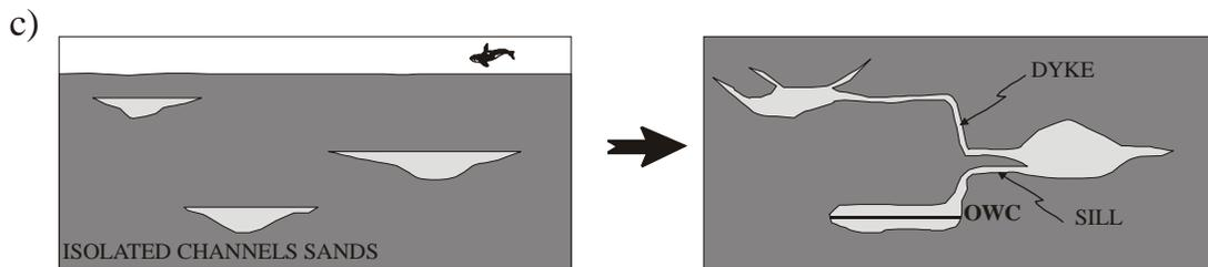
CHANGE IN CONNECTIVITY OF ORIGINALLY ISOLATED RESERVOIRS
