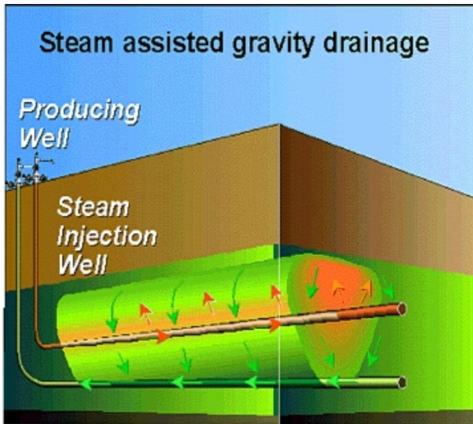
**Figure 2.** Schematic of a SAGD Well pair. Steam is injected in the upper horizontal well with the hot bitumen produced from the lower well.
