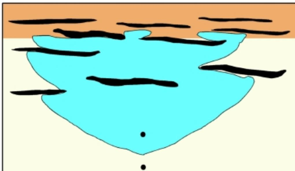
**Figure 3.** Schematic picture of a steam chamber in a heterolithic reservoir. Note how the steam chamber goes around the edges of discontinuous shale barriers but the upper, more continuous shale beds are effective at limiting further steam rise.
