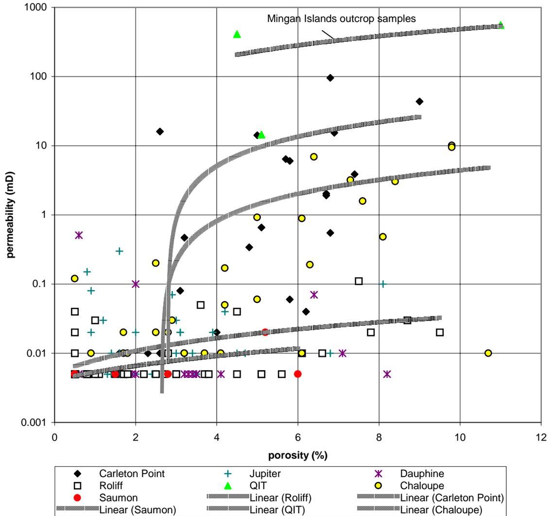
**Figure 4.** Sidewall core porosity-permeability data demonstrating enhanced permeability within Romaine Formation rocks affected by dolomite dissolution (de-dolomitization) such as at Carleton Point, Chaloupe, and QIT quarry (Mingan Islands); other samples do not show evidence of de-dolomitization and have corresponding low-permeabilities.
