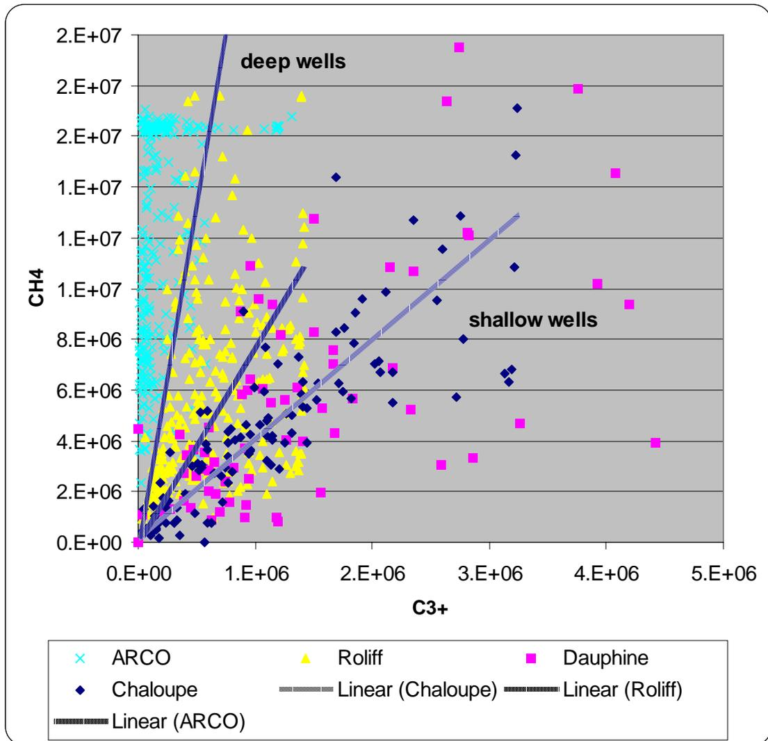
**Figure 2.** Bulk fluid inclusion analyses from cuttings for wells on Anticosti Island, indicating tendency of deep wells to be gas prone and shallow wells to be oil prone. Samples collected from Romaine, Mingan, and Trenton formations.
