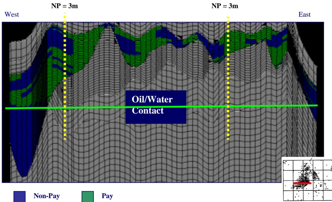
**Figure 4:** Structural cross-section from 3D geological model. The highlighted horizon is the bioturbated channel-fill facies. Based on cut-offs imposed to determine minimum reservoir quality in this facies, the green highlighted cells represent reservoir quality rock with this facies (above the oil/water contact). Blue highlighted cells represent non-reservoir quality rock, above the oil/water contact. Note that the extreme variability is based on 200 to 400m well spacing.
