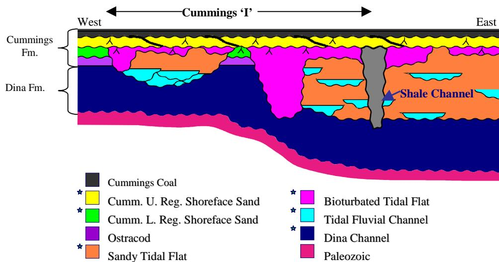
**Figure 2:** Cross-sectional cartoon of the Cummings 'I' pool. The pool is comprised of six reservoir facies found in three interpreted fluvial-estuarine channels and two shorefaces. The pool is trapped by an updip shale channel and sealed by an overlying paleosol and coal sequence. Asterisks denote reservoir units.
