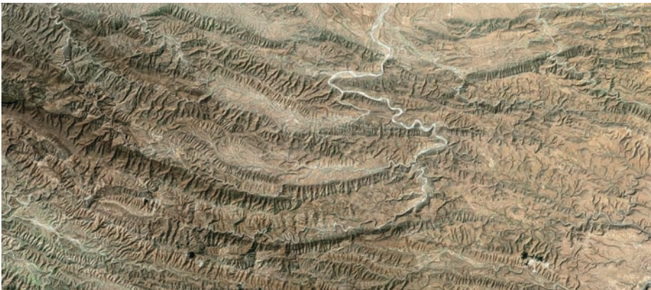
Figure 7. Gulf of Aden rift margin, Somalia. Drainage patterns preferentially exploit relay ramps. The view is 50 km across.
