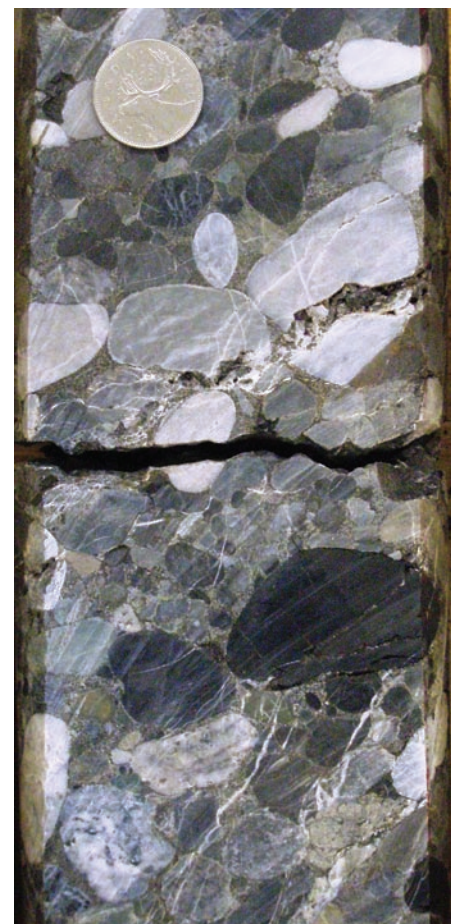
Figure 2. Poorly sorted Cadomin conglomerate with sandy matrix. Extensive silicification has almost completely destroyed primary matrix porosity. Brittle fractures (some filled) provide some overall permeability to the Cadomin reservoir.
