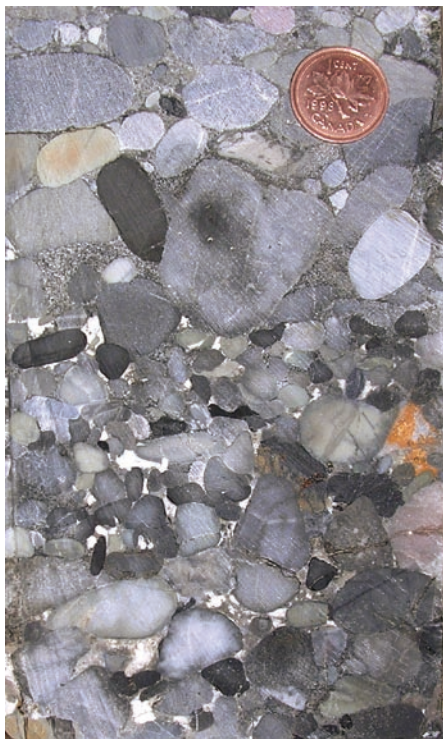
Figure 3. Cadomin conglomerate – some interpebble porosity occurs where sandy matrix is absent, but it has been largely filled by white authigenic clay.
