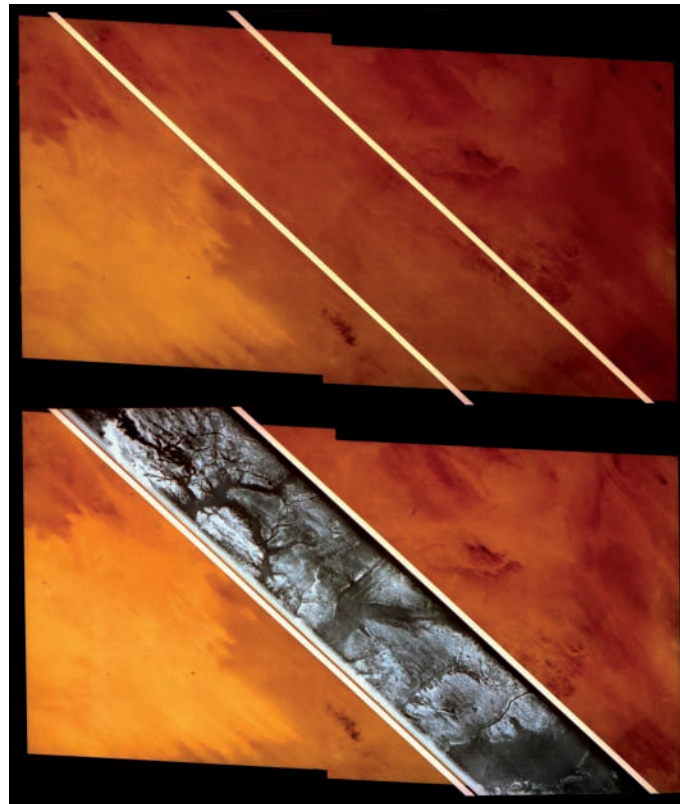
Figure 4. Top shows visible image of eastern Sahara. Strip on bottom shows long-wavelength Radar image revealing ancient river channels (dark) (source: JPL/NASA).
