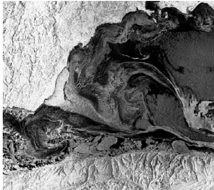
Figure 2. Radarsat 1 image of the Gulf of St. Lawrence showing ice and current formations. Radar images have one band only, so appear as grey scale (source: Canadian Space Agency 2005).
