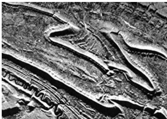
Figure 3. Geological structure (synclines in Pennsylvania) highlighted by radar shadows. This effect works equally well for exposed rock, vegetation-covered rock, and on extraterrestrial bodies (source: Natural Resources Canada).
