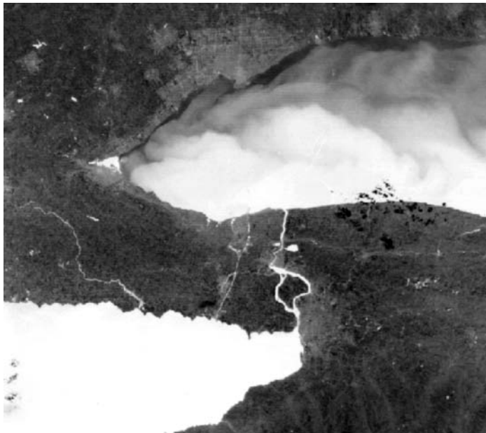
Figure 1. Landsat night-time tir image showing Lakes Erie and Ontario, including Buffalo and Toronto. Warmer temperatures show as lighter tones. Direction of flow of the Niagara River (centre) from south (the warmer L. Erie) to north (cooler L. Ontario) is evident. Currents in L. Ontario and Toronto's cold waterfront show up well. The black specks centre right are (cold) clouds (source: NASA http://rst.gsfc.nasa.gov/Sect9/Sect9_6.html ).
