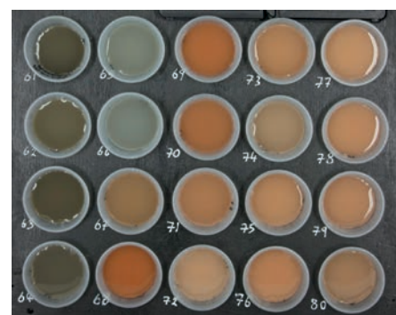
Figure 4. Example of saturated sample slurries illustrating the readily observable changes captured by our sampling methodology. Even in a seemingly homogenous section of black and neutral colored samples, significant changes and gradations are evident. Here, downhole depths increase top to bottom and left to right.
