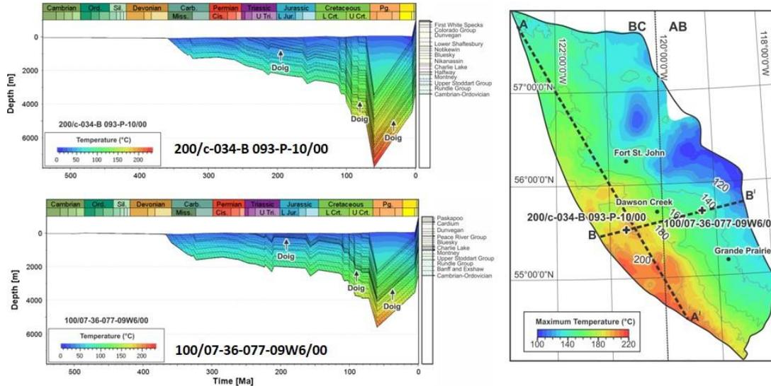
Figure 1: Left - Basin subsidence history of the WCSB at the two locations shown on the map; right - Maximum temperature map of the Doig Formation, with locations of subsidence history diagrams and cross-sections in Figure 2.
